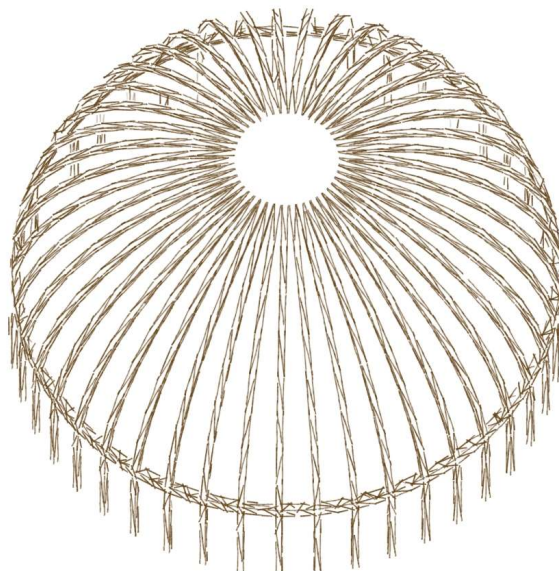
Illustration 4: 40 chevrons forment la coupole
